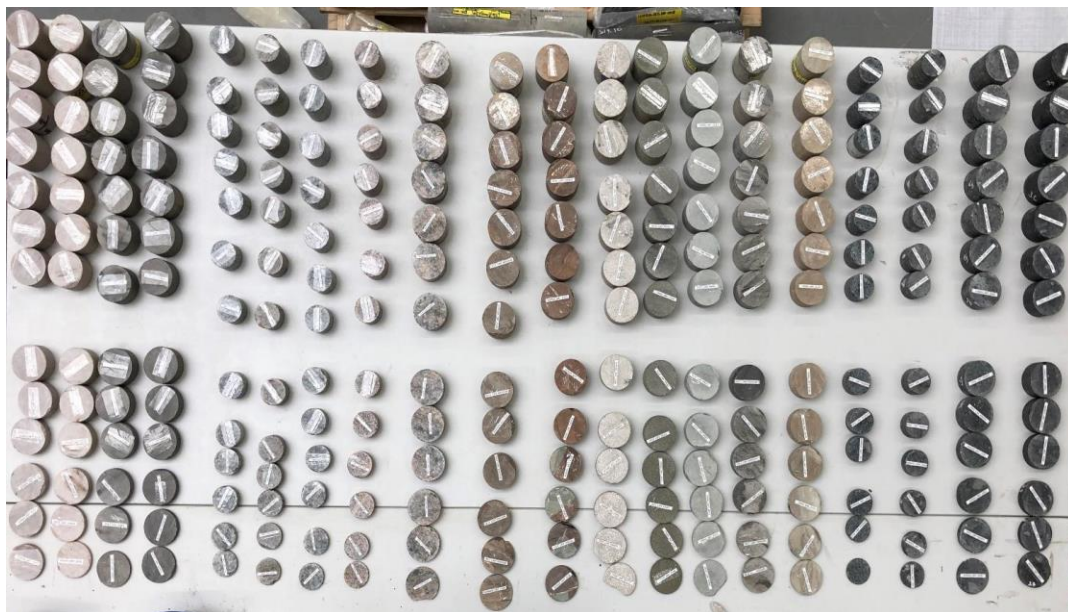
Figure 13-1: Ore and Waste Samples Prepared for XRT Testing
